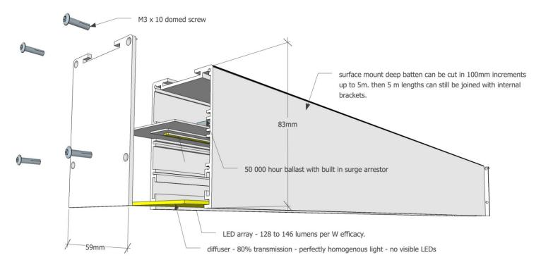
Lumen values are as measured at source - on the PCB - not exiting light fitting. Due to the fast pace of development - values are subject to change at any time and without notice.
