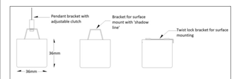
Up to 5000mm in a single length – opal diffuser size is 2400mm in one piece maximum. Lengths can be joined to make longer lengths
