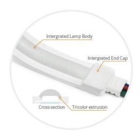
IP 65 version - with a UV stable silicone sheath that is not bonded or glued to the PCB – allowing for expansion and contraction in sunlight – without putting strain on the electronics within. Frosted lens presents a constant bead of light - no dots.
